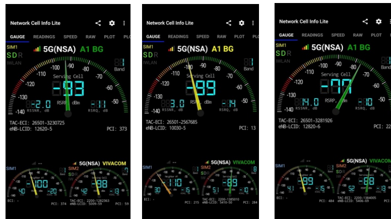
Fig 4.76. Signal power, information about the serving cell, neighboring cells and the second SIM card
