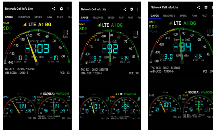
Fig 4.61. Signal strength, information about the cell in use, neighboring cells and the second SIM card
