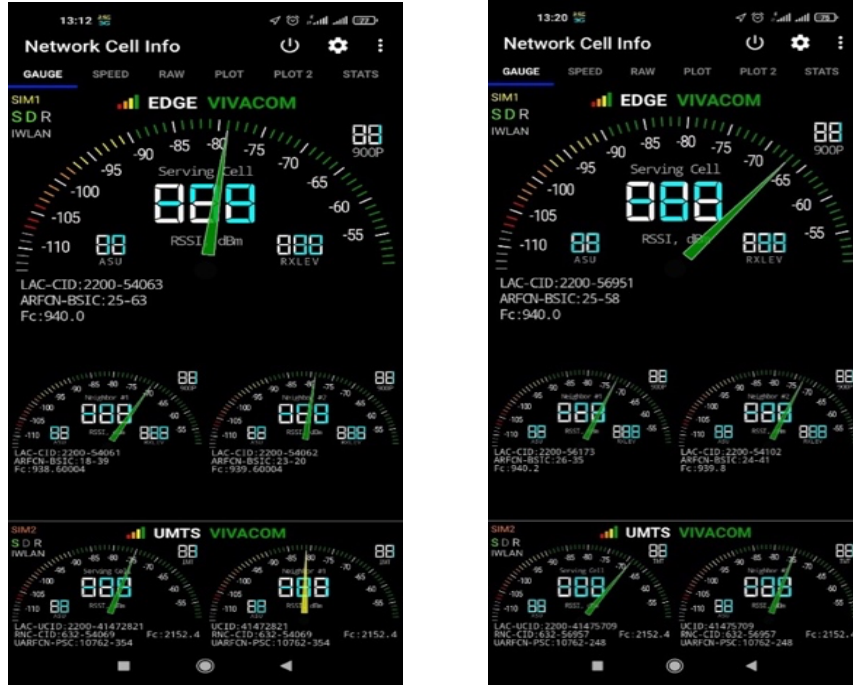
Fig. 4.6. Signal power information about the cell in use, neighboring cells and the second SIM card
