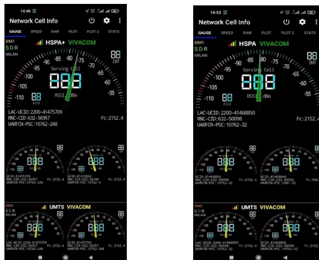
Fig. 4.21. Signal strength, information about the cell in use, neighboring cells and the second SIM card
