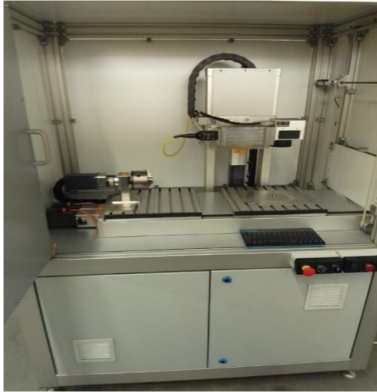
Fig.2.3. General view of the laser marking system for layered reinforced composites with a polymer matrix
