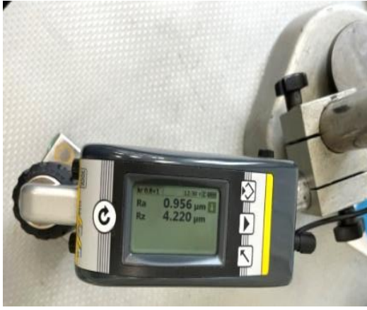
Fig.3.5. Scheme of roughness measurement by criterion, Ra , \mu m .
